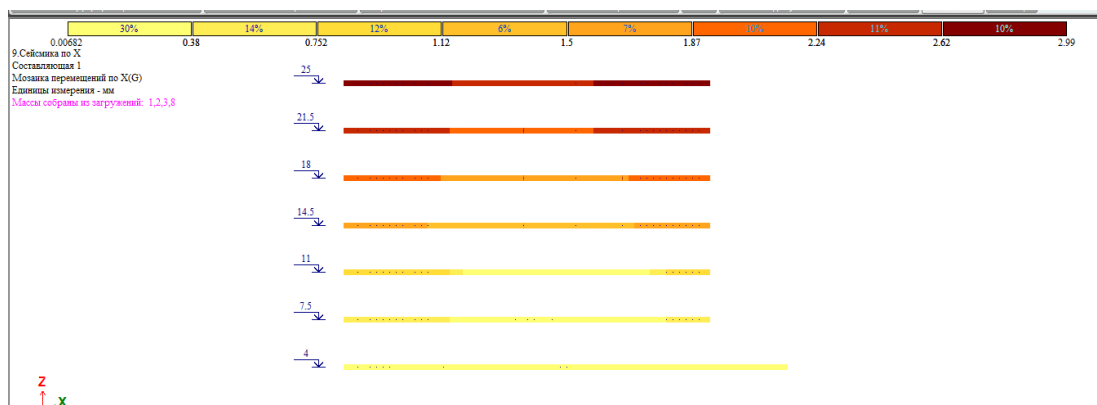
Figure 2.21 - Displacement of ceilings from seismic actions along the X axis
