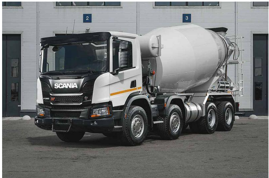
Figure 3.5 – SCANIA concrete mixer
