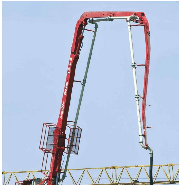
Figure 3.4 – BHD 19+3 concrete distribution boom
